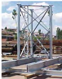
Lattice and polygonal type antenna poles for building roofs.
